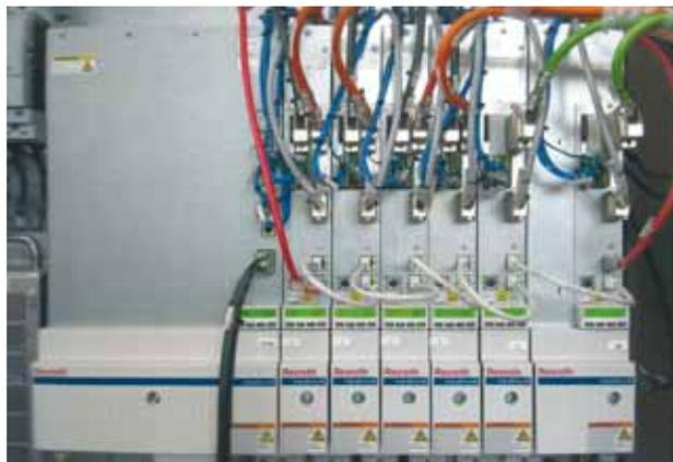
With regard to speed, although the first generation of sercos was very good in this respect, the latest generation is even better. With the third generation of the sercos Motion Control profile, it is now possible to whittle sampling cycle times down to 0.5 milliseconds. This time determines machine performance, i.e. the machine has become even more precise.
