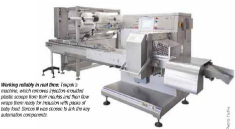
machine, which removes injection-moulded plastic scoops from their moulds and then flow wraps them ready for inclusion with packs of baby food. Sercos III was chosen to link the key automation components.
