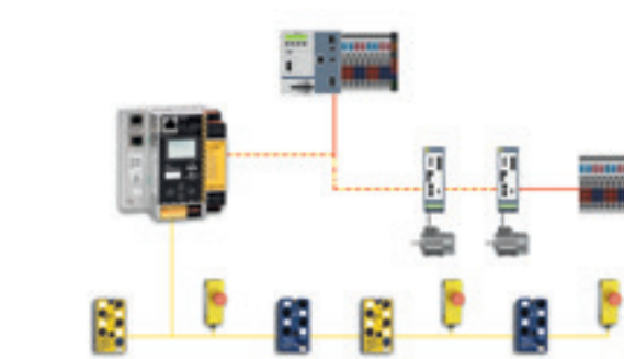
AS-i Safety Gateway used as a CIP Safety Originator in the Sercos network without an additional safety controller. This allows the advantages of AS-i and AS-i Safety to be exploited in parallel on the lowest field level.
